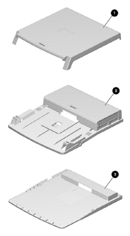
Figure 3-10. MultiBay Expansion Base Cover Assemblies
